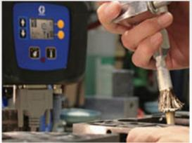
Instead, a sensor tracks the pump position so that the pump acts like a flowmeter. The amount dispensed is based on pump size.
