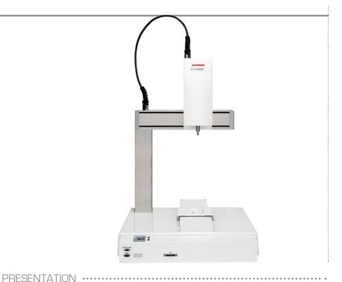
With its large working area of 400 x 400 mm, the JR2400N dispensing robot takes less than 629 mm<sup>2</sup> workspace. This robot has an opening on the side for easy handling unhardy objects in and around the work area.
